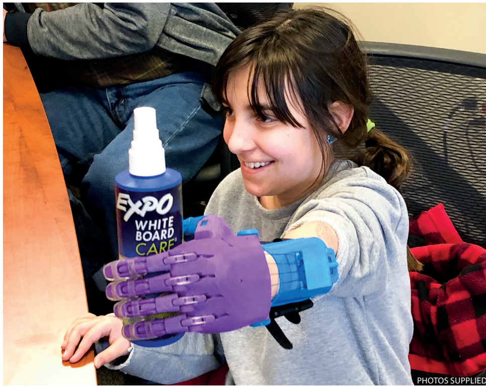
Jerlana Rittwage, who is missing her left hand, has a new prosthetic hand thanks to high school students Jonas Prudden (blue hoodie) and Levi Schmidtke. The hand is controlled by wrist movements.
